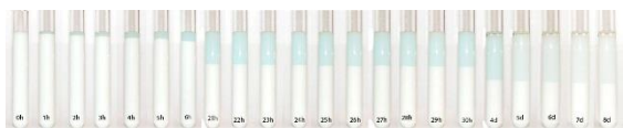
Figure 15 - Evolution of the emulsion using 6g of SPAN 80, from 0 hours to 8 days
